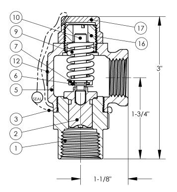
Inlet Sizes 1/4" - 3/8" - 1/2" Outlet Size 1/2" Max Temp: 406°F Max Pressure: 200 P.S.I.
