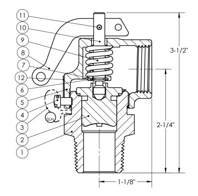
Safety Valve - Air / Gas / Steam ASME - NB Section XIII "UV" for Section VIII Div. 1, CRN
